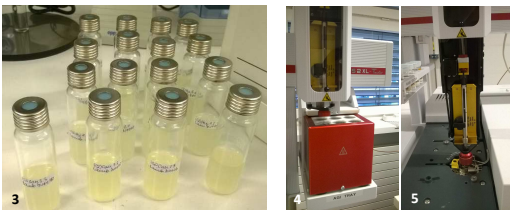
3. 8 mL yeast culture sampled into glass vials ready to be frozen at -80 °C and then utilized for GC-MS analyses. 4. and 5. Equipment utilized in the Unibz laboratories for the analyses of volatile compounds with DHS-GC-MS: GC-MS (7890A-5975C, Agilent Technologies, Santa Clara, USA) with incubator/shaker and multipurpose autosampler (Gerstel, Mülheim an der Ruhr, Germany).
