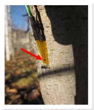
Fig. 1: A temperature sensor prior to (left) and after insertion (right) under the tree bark. The red arrow indicates the sensor's exact measuring
